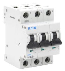
Eaton miniature supplementary protector, 30A, 480Y / 277 VAC / 96 VDC, 3-pole, D curve, thermal magnetic, 5kA @ 480Y/277 VAC interrupting rating, 35mm DIN rail mount.
