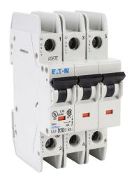
Eaton miniature circuit breaker, current-limiting, 30A, 240 VAC / 96 VDC, 3-pole, D curve, thermal magnetic, 10kA @ 240 VAC interrupting rating, 35mm DIN rail mount.
