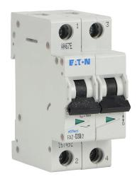
Eaton miniature supplementary protector, 30A, 480Y / 277 VAC / 96 VDC, 2-pole, D curve, thermal magnetic, 5kA @ 480Y/277 VAC interrupting rating, 35mm DIN rail mount.
