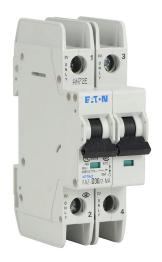
Eaton miniature circuit breaker, current-limiting, 30A, 480Y / 277 VAC / 96 VDC, 2-pole, D curve, thermal magnetic, 10kA @ 480Y/277 VAC interrupting rating, 35mm DIN rail mount.
