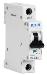
Eaton miniature supplementary protector, 30A, 277 VAC / 48 VDC, 1-pole, D curve, thermal magnetic, 5kA @ 277 VAC interrupting rating, 35mm DIN rail mount.
