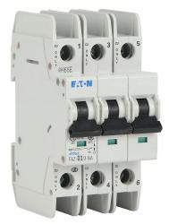
Eaton miniature circuit breaker, current-limiting, 3A, 480Y / 277 VAC / 96 VDC, 3-pole, D curve, thermal magnetic, 10kA @ 480Y/277 VAC interrupting rating, 35mm DIN rail mount.
