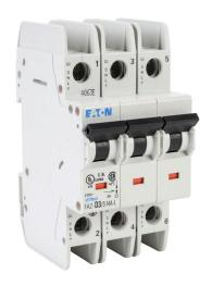
Eaton miniature circuit breaker, current-limiting, 3A, 240 VAC / 96 VDC, 3-pole, D curve, thermal magnetic, 10kA @ 240 VAC interrupting rating, 35mm DIN rail mount.
