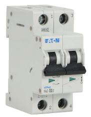
Eaton miniature supplementary protector, 3A, 480Y / 277 VAC / 96 VDC, 2-pole, D curve, thermal magnetic, 5kA @ 480Y/277 VAC interrupting rating, 35mm DIN rail mount.
