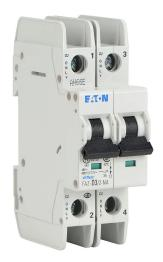
Eaton miniature circuit breaker, current-limiting, 3A, 480Y / 277 VAC / 96 VDC, 2-pole, D curve, thermal magnetic, 10kA @ 480Y/277 VAC interrupting rating, 35mm DIN rail mount.
