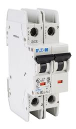
Eaton miniature circuit breaker, current-limiting, 3A, 240 VAC / 96 VDC, 2-pole, D curve, thermal magnetic, 10kA @ 240 VAC interrupting rating, 35mm DIN rail mount.
