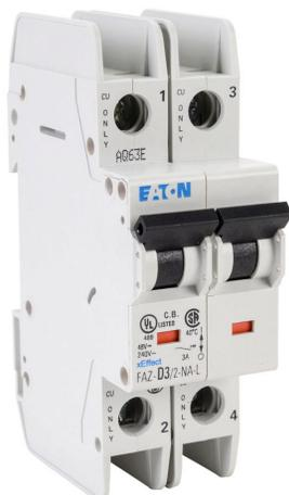
Eaton miniature circuit breaker, current-limiting, 3A, 240 VAC / 96 VDC, 2-pole, D curve, thermal magnetic, 10kA @ 240 VAC interrupting rating, 35mm DIN rail mount.
