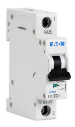
Eaton miniature supplementary protector, 3A, 277 VAC / 48 VDC, 1-pole, D curve, thermal magnetic, 5kA @ 277 VAC interrupting rating, 35mm DIN rail mount.
