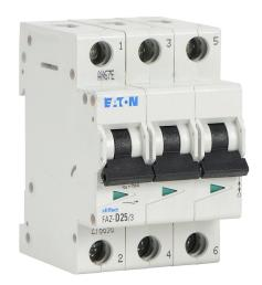
Eaton miniature supplementary protector, 25A, 480Y / 277 VAC / 96 VDC, 3-pole, D curve, thermal magnetic, 5kA @ 480Y/277 VAC interrupting rating, 35mm DIN rail mount.
