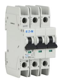
Eaton miniature circuit breaker, current-limiting, 25A, 480Y / 277 VAC / 96 VDC, 3-pole, D curve, thermal magnetic, 10kA @ 480Y/277 VAC interrupting rating, 35mm DIN rail mount.
