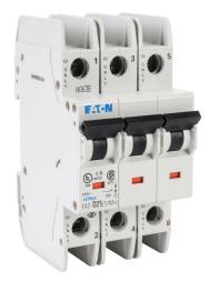
Eaton miniature circuit breaker, current-limiting, 25A, 240 VAC / 96 VDC, 3-pole, D curve, thermal magnetic, 10kA @ 240 VAC interrupting rating, 35mm DIN rail mount.
