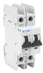
Eaton miniature circuit breaker, current-limiting, 25A, 480Y / 277 VAC / 96 VDC, 2-pole, D curve, thermal magnetic, 10kA @ 480Y/277 VAC interrupting rating, 35mm DIN rail mount.
