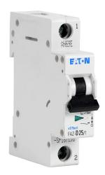
Eaton miniature supplementary protector, 25A, 277 VAC / 48 VDC, 1-pole, D curve, thermal magnetic, 5kA @ 277 VAC interrupting rating, 35mm DIN rail mount.
