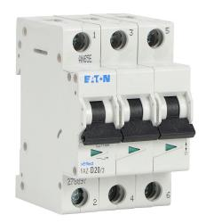
Eaton miniature supplementary protector, 20A, 480Y / 277 VAC / 96 VDC, 3-pole, D curve, thermal magnetic, 5kA @ 480Y/277 VAC interrupting rating, 35mm DIN rail mount.
