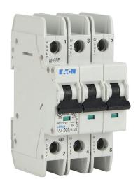
Eaton miniature circuit breaker, current-limiting, 20A, 480Y / 277 VAC / 96 VDC, 3-pole, D curve, thermal magnetic, 14kA @ 480Y/277 VAC interrupting rating, 35mm DIN rail mount.
