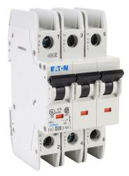
Eaton miniature circuit breaker, current-limiting, 20A, 240 VAC / 96 VDC, 3-pole, D curve, thermal magnetic, 14kA @ 240 VAC interrupting rating, 35mm DIN rail mount.
