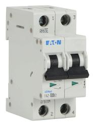
Eaton miniature supplementary protector, 20A, 480Y / 277 VAC / 96 VDC, 2-pole, D curve, thermal magnetic, 5kA @ 480Y/277 VAC interrupting rating, 35mm DIN rail mount.
