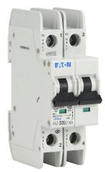
Eaton miniature circuit breaker, current-limiting, 20A, 480Y / 277 VAC / 96 VDC, 2-pole, D curve, thermal magnetic, 14kA @ 480Y/277 VAC interrupting rating, 35mm DIN rail mount.
