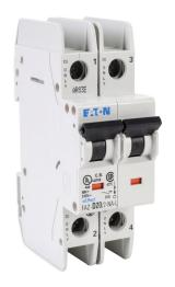
Eaton miniature circuit breaker, current-limiting, 20A, 240 VAC / 96 VDC, 2-pole, D curve, thermal magnetic, 14kA @ 240 VAC interrupting rating, 35mm DIN rail mount.
