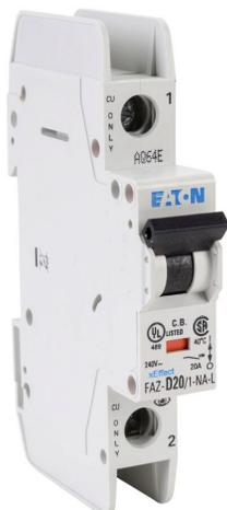
Eaton miniature circuit breaker, current-limiting, 20A, 240 VAC / 48 VDC, 1-pole, D curve, thermal magnetic, 14kA @ 240 VAC interrupting rating, 35mm DIN rail mount.
