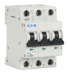
Eaton miniature supplementary protector, 2A, 480Y / 277 VAC / 96 VDC, 3-pole, D curve, thermal magnetic, 5kA @ 480Y/277 VAC interrupting rating, 35mm DIN rail mount.
