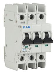
Eaton miniature circuit breaker, current-limiting, 2A, 480Y / 277 VAC / 96 VDC, 3-pole, D curve, thermal magnetic, 10kA @ 480Y/277 VAC interrupting rating, 35mm DIN rail mount.
