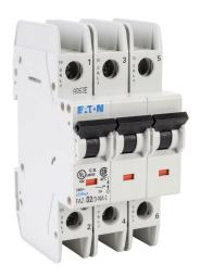
Eaton miniature circuit breaker, current-limiting, 2A, 240 VAC / 96 VDC, 3-pole, D curve, thermal magnetic, 10kA @ 240 VAC interrupting rating, 35mm DIN rail mount.
