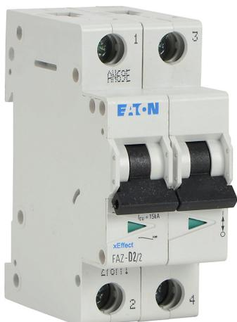
Eaton miniature supplementary protector, 2A, 480Y / 277 VAC / 96 VDC, 2-pole, D curve, thermal magnetic, 5kA @ 480Y/277 VAC interrupting rating, 35mm DIN rail mount.
