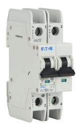
Eaton miniature circuit breaker, current-limiting, 2A, 480Y / 277 VAC / 96 VDC, 2-pole, D curve, thermal magnetic, 10kA @ 480Y/277 VAC interrupting rating, 35mm DIN rail mount.
