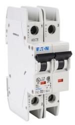
Eaton miniature circuit breaker, current-limiting, 2A, 240 VAC / 96 VDC, 2-pole, D curve, thermal magnetic, 10kA @ 240 VAC interrupting rating, 35mm DIN rail mount.
