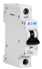
Eaton miniature supplementary protector, 2A, 277 VAC / 48 VDC, 1-pole, D curve, thermal magnetic, 5kA @ 277 VAC interrupting rating, 35mm DIN rail mount.
