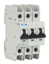
Eaton miniature circuit breaker, current-limiting, 1.5A, 480Y / 277 VAC / 96 VDC, 3-pole, D curve, thermal magnetic, 10kA @ 480Y/277 VAC interrupting rating, 35mm DIN rail mount.
