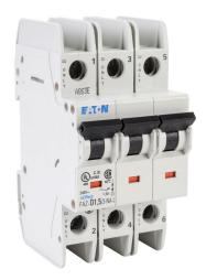
Eaton miniature circuit breaker, current-limiting, 1.5A, 240 VAC / 96 VDC, 3-pole, D curve, thermal magnetic, 10kA @ 240 VAC interrupting rating, 35mm DIN rail mount.
