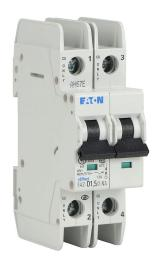
Eaton miniature circuit breaker, current-limiting, 1.5A, 480Y / 277 VAC / 96 VDC, 2-pole, D curve, thermal magnetic, 10kA @ 480Y/277 VAC interrupting rating, 35mm DIN rail mount.
