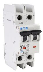
Eaton miniature circuit breaker, current-limiting, 1.5A, 240 VAC / 96 VDC, 2-pole, D curve, thermal magnetic, 10kA @ 240 VAC interrupting rating, 35mm DIN rail mount.
