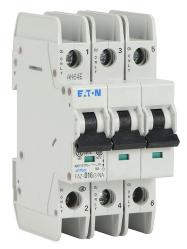
Eaton miniature circuit breaker, current-limiting, 16A, 480Y / 277 VAC / 96 VDC, 3-pole, D curve, thermal magnetic, 14kA @ 480Y/277 VAC interrupting rating, 35mm DIN rail mount.
