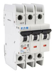
Eaton miniature circuit breaker, current-limiting, 16A, 240 VAC / 96 VDC, 3-pole, D curve, thermal magnetic, 14kA @ 240 VAC interrupting rating, 35mm DIN rail mount.
