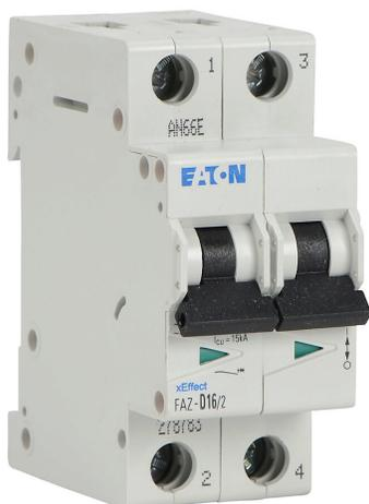
Eaton miniature supplementary protector, 16A, 480Y / 277 VAC / 96 VDC, 2-pole, D curve, thermal magnetic, 5kA @ 480Y/277 VAC interrupting rating, 35mm DIN rail mount.
