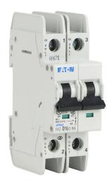
Eaton miniature circuit breaker, current-limiting, 16A, 480Y / 277 VAC / 96 VDC, 2-pole, D curve, thermal magnetic, 14kA @ 480Y/277 VAC interrupting rating, 35mm DIN rail mount.
