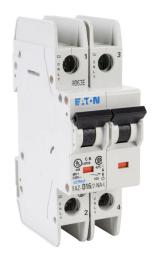
Eaton miniature circuit breaker, current-limiting, 16A, 240 VAC / 96 VDC, 2-pole, D curve, thermal magnetic, 14kA @ 240 VAC interrupting rating, 35mm DIN rail mount.
