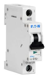
Eaton miniature supplementary protector, 16A, 277 VAC / 48 VDC, 1-pole, D curve, thermal magnetic, 5kA @ 277 VAC interrupting rating, 35mm DIN rail mount.
