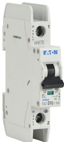
Eaton miniature circuit breaker, current-limiting, 16A, 277 VAC / 48 VDC, 1-pole, D curve, thermal magnetic, 14kA @ 277 VAC interrupting rating, 35mm DIN rail mount.
