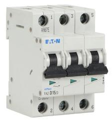
Eaton miniature supplementary protector, 15A, 480Y / 277 VAC / 96 VDC, 3-pole, D curve, thermal magnetic, 5kA @ 480Y/277 VAC interrupting rating, 35mm DIN rail mount.
