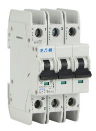
Eaton miniature circuit breaker, current-limiting, 15A, 480Y / 277 VAC / 96 VDC, 3-pole, D curve, thermal magnetic, 14kA @ 480Y/277 VAC interrupting rating, 35mm DIN rail mount.
