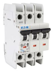
Eaton miniature circuit breaker, current-limiting, 15A, 240 VAC / 96 VDC, 3-pole, D curve, thermal magnetic, 14kA @ 240 VAC interrupting rating, 35mm DIN rail mount.
