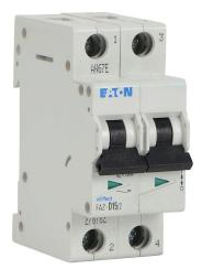
Eaton miniature supplementary protector, 15A, 480Y / 277 VAC / 96 VDC, 2-pole, D curve, thermal magnetic, 5kA @ 480Y/277 VAC interrupting rating, 35mm DIN rail mount.
