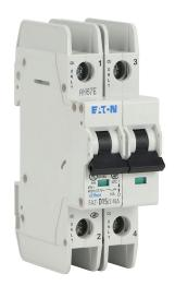
Eaton miniature circuit breaker, current-limiting, 15A, 480Y / 277 VAC / 96 VDC, 2-pole, D curve, thermal magnetic, 14kA @ 480Y/277 VAC interrupting rating, 35mm DIN rail mount.
