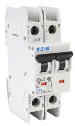
Eaton miniature circuit breaker, current-limiting, 15A, 240 VAC / 96 VDC, 2-pole, D curve, thermal magnetic, 14kA @ 240 VAC interrupting rating, 35mm DIN rail mount.
