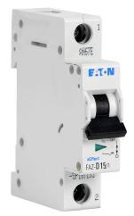
Eaton miniature supplementary protector, 15A, 277 VAC / 48 VDC, 1-pole, D curve, thermal magnetic, 5kA @ 277 VAC interrupting rating, 35mm DIN rail mount.
