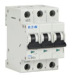
Eaton miniature supplementary protector, 13A, 480Y / 277 VAC / 96 VDC, 3-pole, D curve, thermal magnetic, 5kA @ 480Y/277 VAC interrupting rating, 35mm DIN rail mount.
