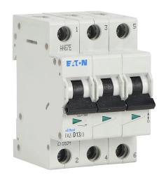
Eaton miniature supplementary protector, 13A, 480Y / 277 VAC / 96 VDC, 3-pole, D curve, thermal magnetic, 5kA @ 480Y/277 VAC interrupting rating, 35mm DIN rail mount.
