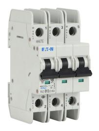
Eaton miniature circuit breaker, current-limiting, 13A, 480Y / 277 VAC / 96 VDC, 3-pole, D curve, thermal magnetic, 14kA @ 480Y/277 VAC interrupting rating, 35mm DIN rail mount.
